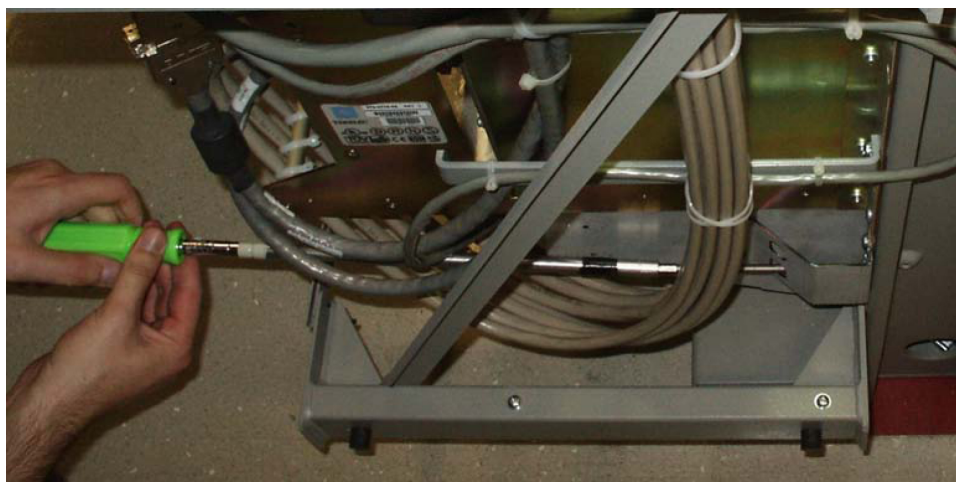
Figure 90: Tighten fan side bracket screws
