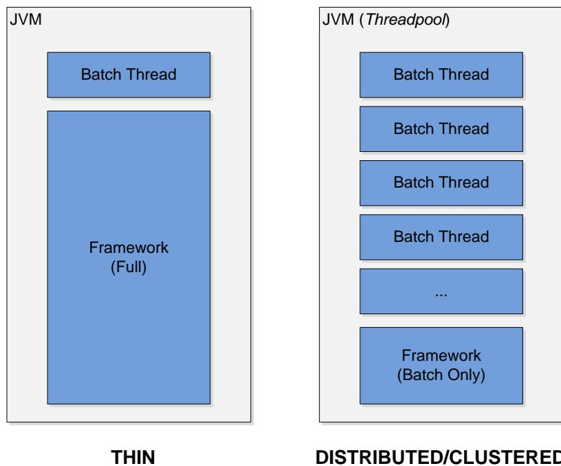
If only **THIN** submissions are ever used, script `threadpoolworker[.sh]` does not have to be executed. If this is the case, batch processes can be submitted in **THIN** mode from the command-line using script `submitjob[.sh]`.
