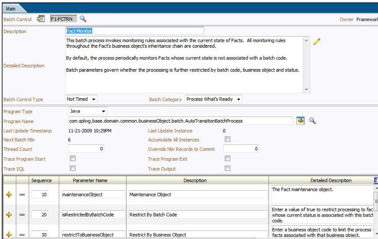
The parameters on the batch control object are:
