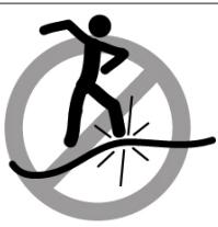
Do not step on the cable or connectors. Plan cable paths away from foot traffic or rolling loads.
