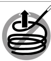
Do not uncoil the cable, as a kink might occur. Hold the coil closed as you unroll the cable, pausing to allow the cable to relax as it is unrolled.
