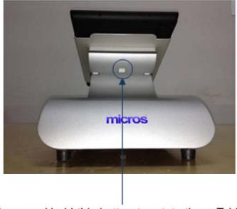
Press and hold this button to rotate the mTablet.
