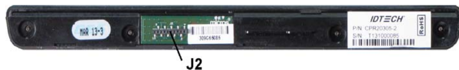
Figure 2-8: Installing the MSR Module
