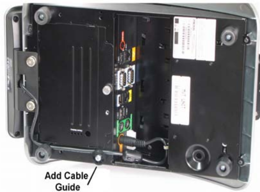
Figure 3-22: Installing the mStation Integrated Customer Display
