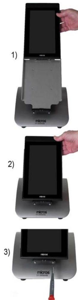
Figure 3-17: Installing the mTablet in mStation - Portrait Mode
