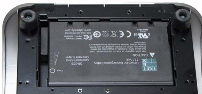
Figure 3-14: Installing the optional mStation Battery Pack
