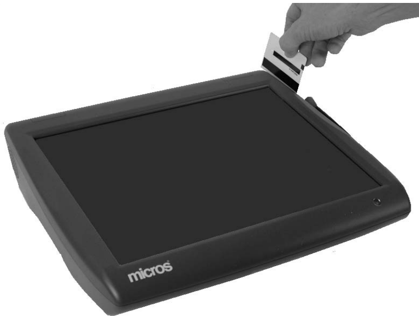
Figure 4-13: Using the Magnetic Card Reader
