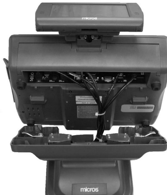
Figure 4-4: Mounting the Workstation to the Adjustable Stand
