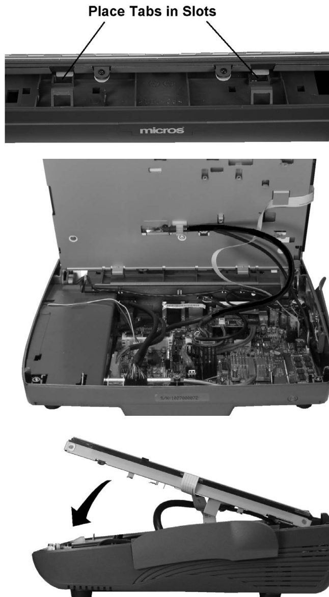
Figure 3-45: Installing the LCD/Touchscreen Assembly
