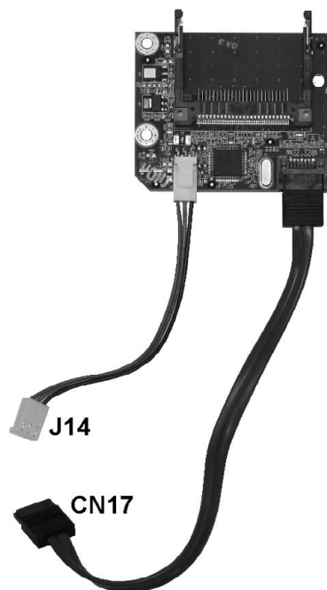
Figure 3-9: SATA CF Riser Card with System Board Cables (Revision C System Board)
