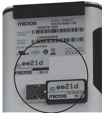
Figure 10: Dongle and Wireless Bump Bar ID labels /w 5-Byte ID
