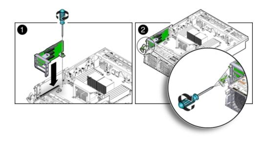
e. Tighten the three green captive Phillips screws that secure the PCIe riser to the chassis [2].
