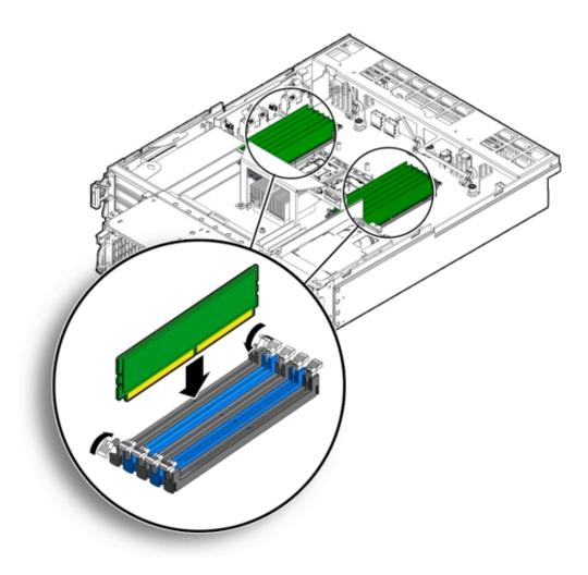
5. Push the DIMM into the connector until the ejector tabs lock the DIMM in place.
