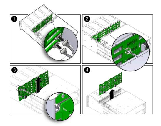
b. Disconnect the two FIM cable connectors from the disk midplane module [1].
