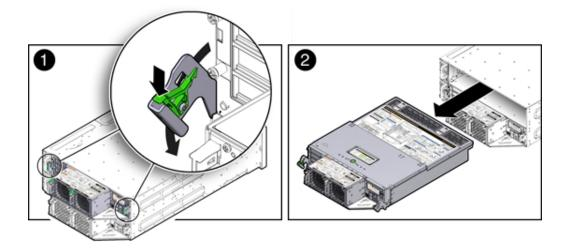
3. Slide the server node to the rear and lift it out of the system [2].
