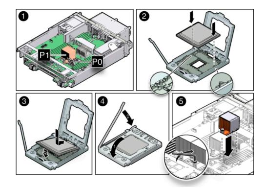
b. Lower the pressure frame to the closed position [4].
