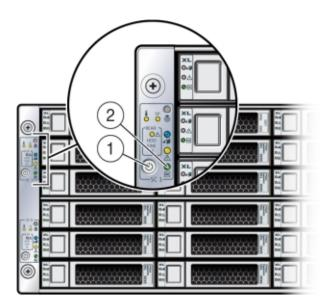
On the server node, the green Power/OK LED [2] blinks while the server node is booting, and remains steady on when the server node is operational.
