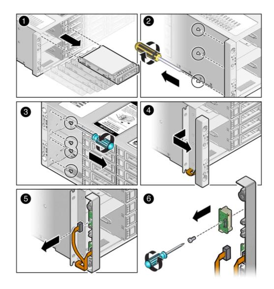
Remove the screw that holds the indicator panel to the ear bezel [6].
