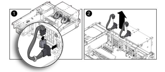
2. Disconnect the fan power cables and remove them from the server node.
