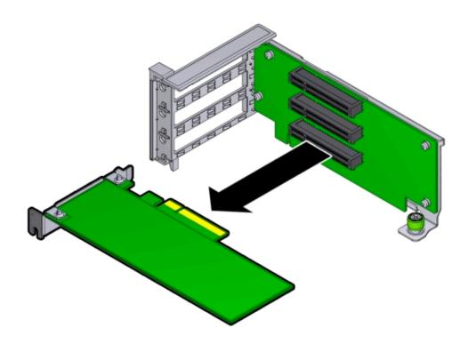
b. Place the PCle card on an antistatic mat.
