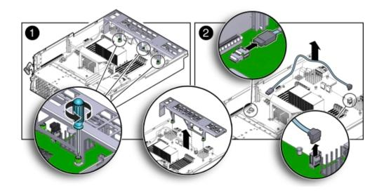
Push the connector inward, press down on the connector to release it, and pull the connector out.
