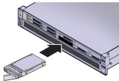
**8. Close the drive latch to lock the drive in place.**
