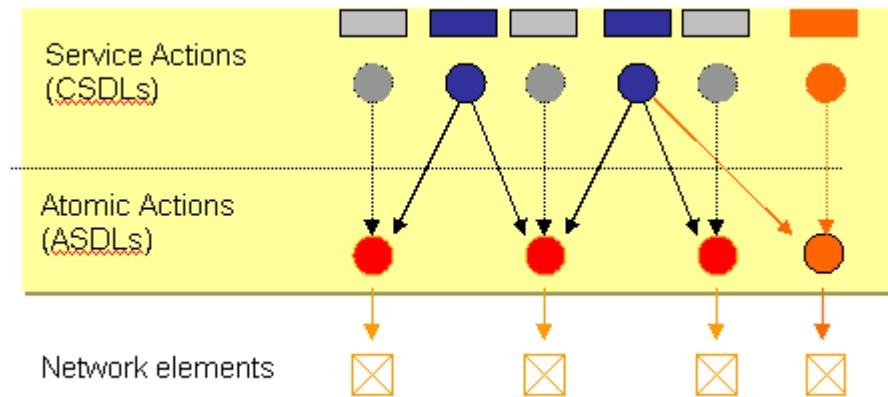
Common service actions (shown in blue) map to multiple vendor, technology, and software load-specific atomic actions (shown in red). The common service actions are shown alongside vendor, technology, and software load-specific service actions from delivered cartridges (in gray) and other solution extensions (shown in orange) that will be discussed in subsequent sections.
