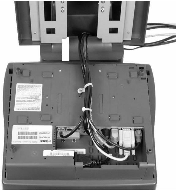
Figure 1-4: Adjustable Stand Cable Management
