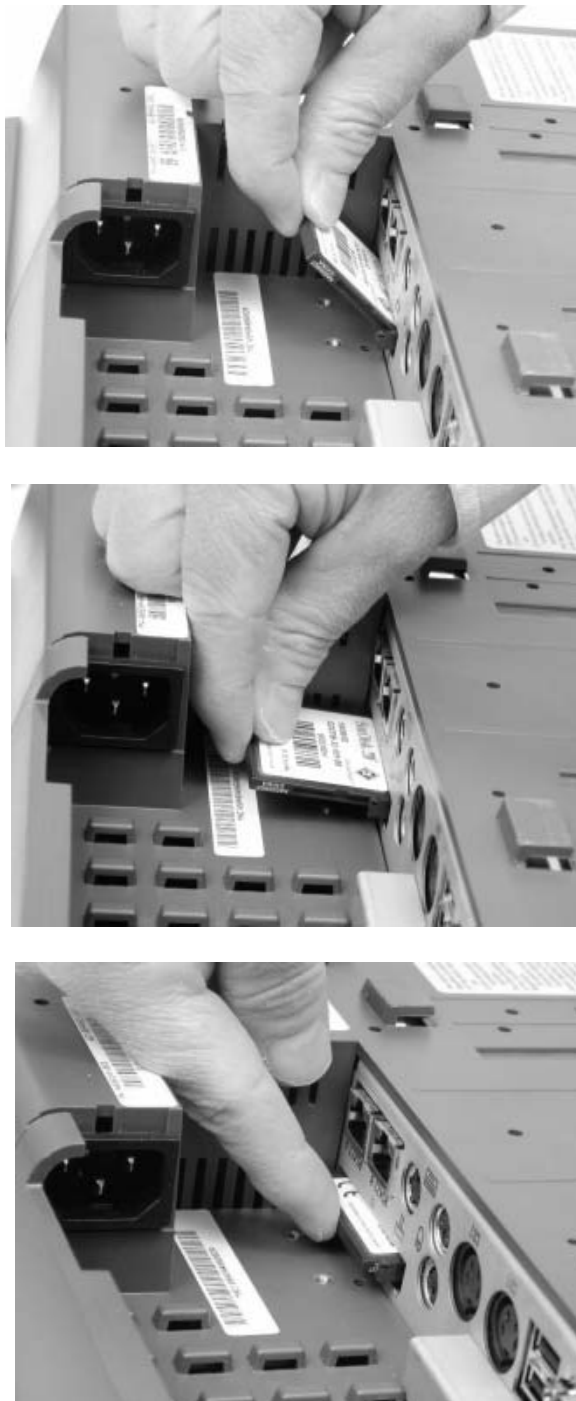
Figure 3-11: Inserting the CF Card
