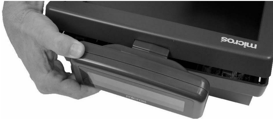
Figure 2-17: Installing the Rear LCD to the Workstation
