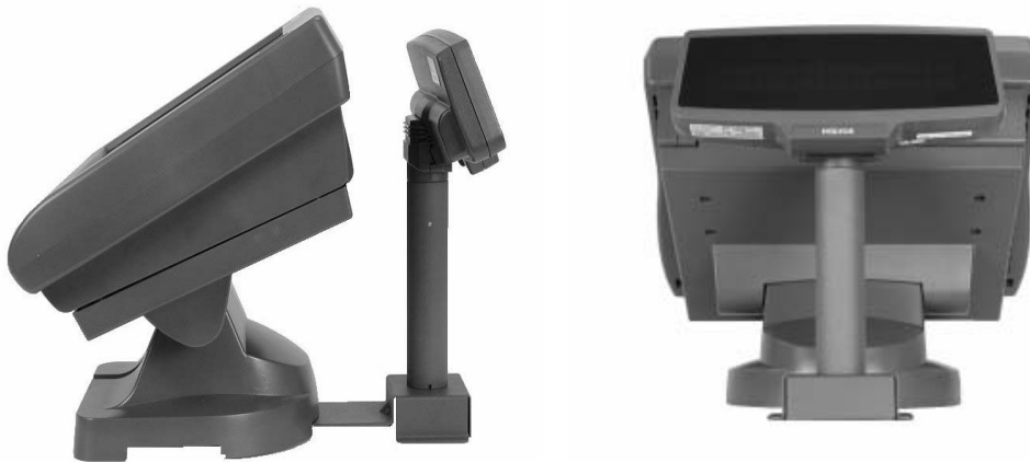
Figure 1-8: VFD Pole Display Mounted to the Adjustable Stand
