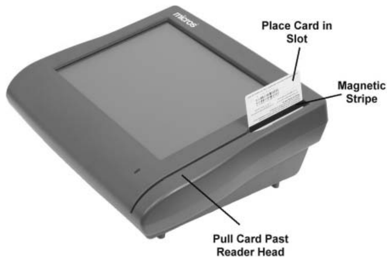
Figure 3-6: Using the Magnetic Card Reader
