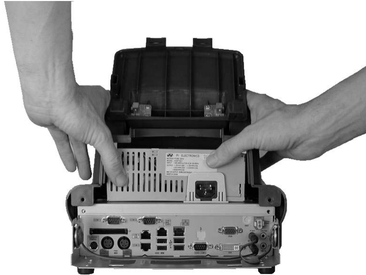
Figure 3-42: Installing the System Unit Cover
