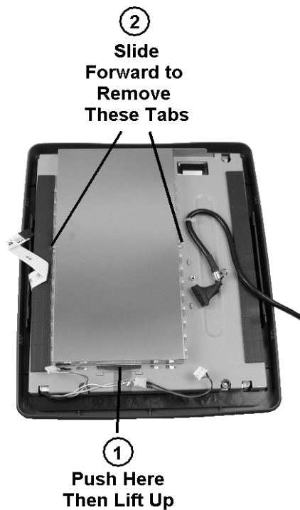
Figure 4-3: Removing the Interface Board Shield
