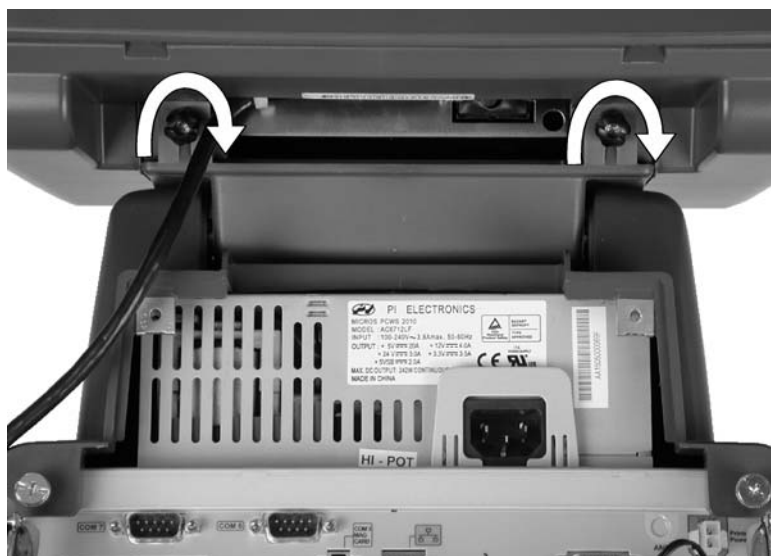
Figure 3-45: Securing the 12.1" LCD/Touchscreen Head to the Pedestal
