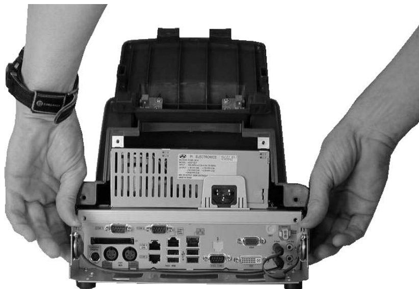
Figure 3-5: Removing the System Unit Cover
