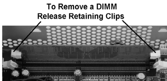
Figure 3-28: Removing a DIMM
