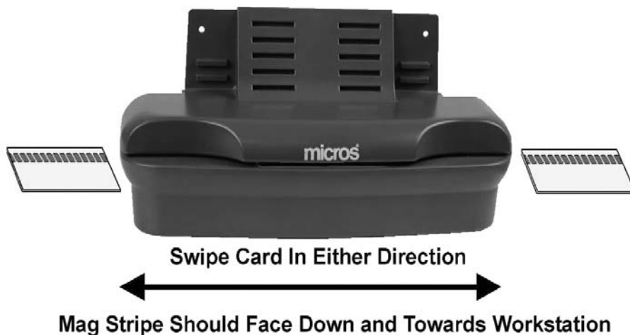
Figure 1-17: Using the Magnetic Card Reader
