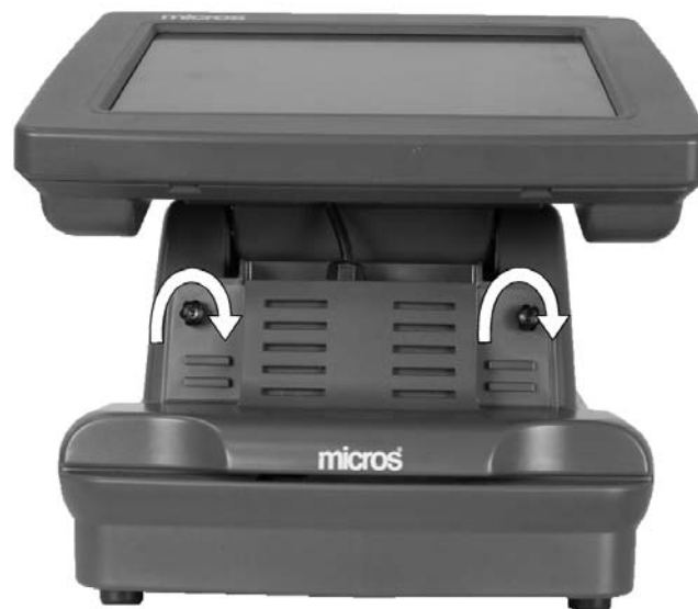
Figure 3-49: Attaching the Front Cover Thumbscrews
