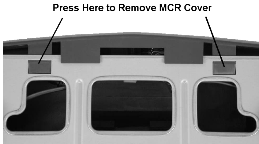
Figure 3-2: Removing the PCWS 2010 MCR Cover
