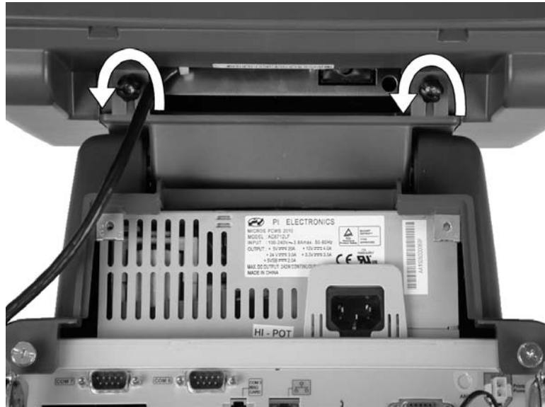
Figure 3-3: Removing the 12.1" LCD/Touchscreen Head
