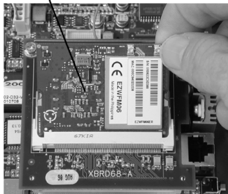
Figure 3: Preparing to install the Mini-PCI Wireless Card
