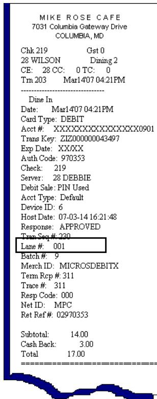
The Pin debit device will maintain the same Lane Number after performing a reboot. Lane Numbers can be changed via the Credit Card Batch Utility by running the Refresh Lane Map function under the *Diagnostics* tab.
