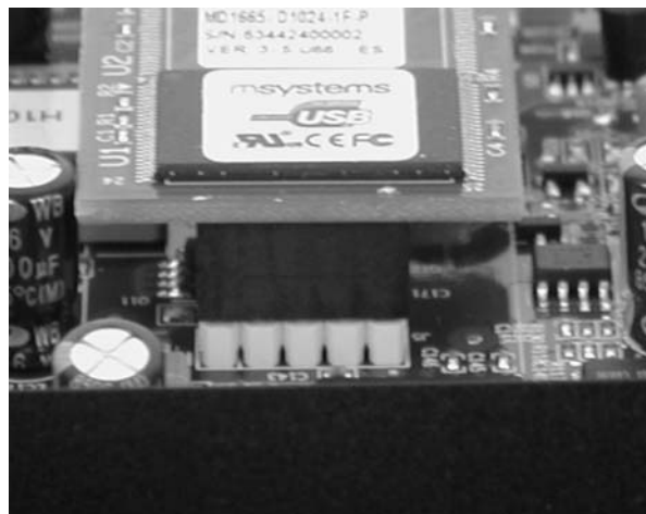
Figure 3-13: Checking the USB Flash Drive Orientation
