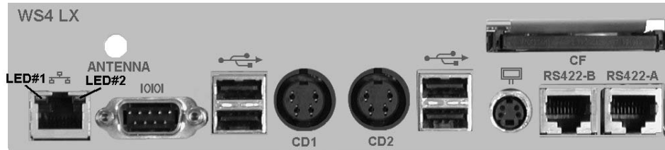
Figure 4-1: Workstation LX 4 I/O Connector Panel
