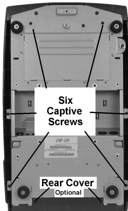
Figure 2-16: Securing the Top Cover to the Chassis
