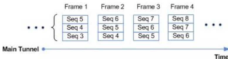
Figure 20-16 Redundancy — DTLS/UDP Redundancy
