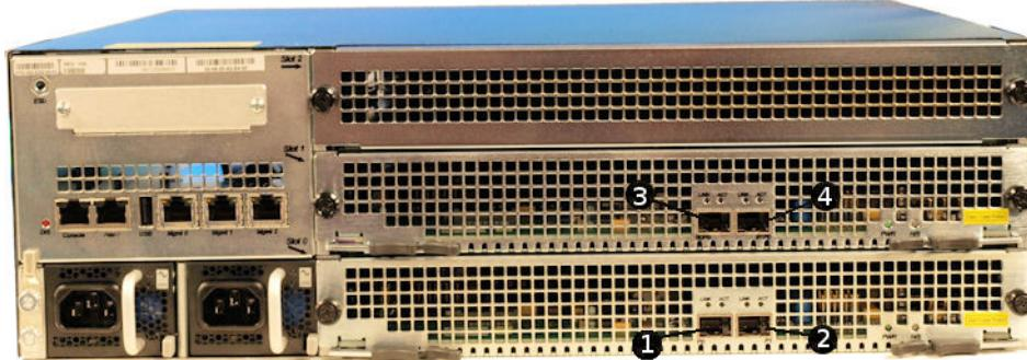
The table below maps the graphic's reference numbers and the labeling on the media interfaces. It also lists the **operation-type**, **slot** and **port** parameters in the **phy-interface** configuration element for the applicable interfaces. Note that the media interfaces are not uniquely labeled with the NIU silkscreen. The table distinguishes between these using "left" and "right", with the perspective being the user looking at the NIU panel.
