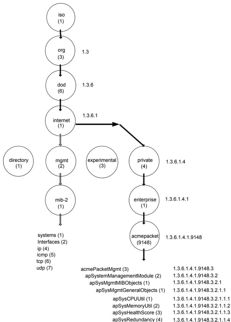
The diagram shows the Acme Packet node has the value 9148; this is Oracle's vendor-specific number that uniquely identifies an Acme Packet product MIB. This node is the highest level of the private (proprietary) branch containing Acme Packet managed objects. The number 9148 was assigned by the Internet Assigned Numbers Authority (IANA).
