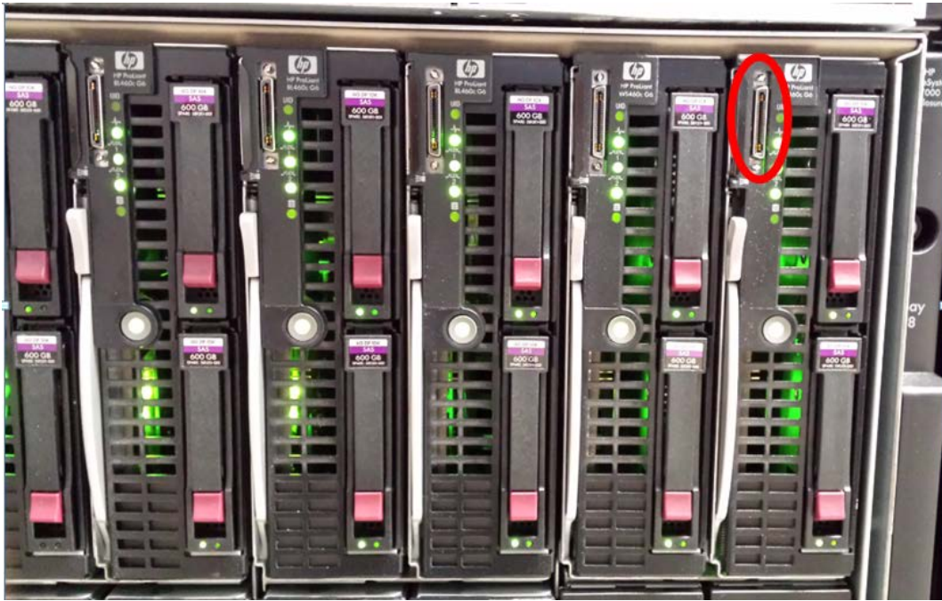
Figure 4: Picture of Front of the Blades showing local terminal connection in the upper left for each blade
