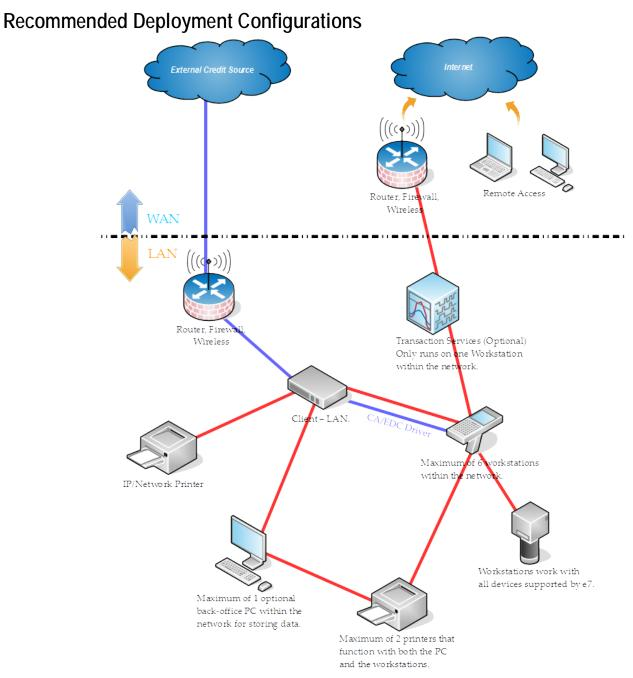
The blue lines represent encrypted credit card transactions to the host. The red lines represent other traffic.
