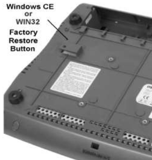
Figure 7 – WS5A Factory Restore Button
