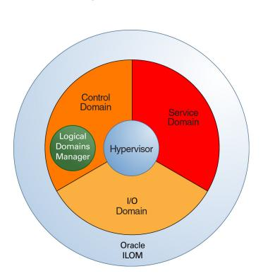
**FIGURE 3** Components of the Execution Environment
