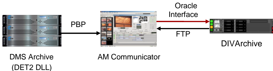
Figure 2: AM Communicator Push Request Processing Workflow
