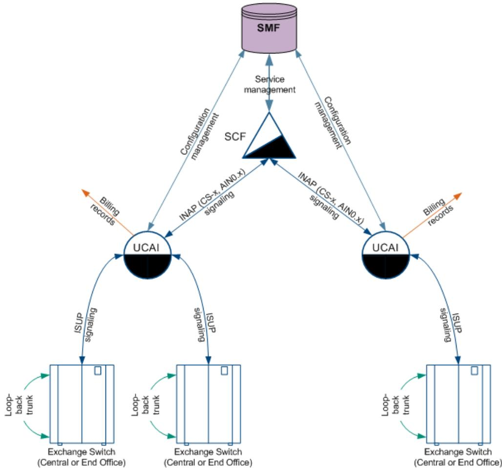
**Note:** Although the UCAI is shown as a separate physical entity in this diagram, it may also co-exist on the SLCs. If so, it will still communicate with the SCF over INAP (though this may not leave the SS7 stack).
