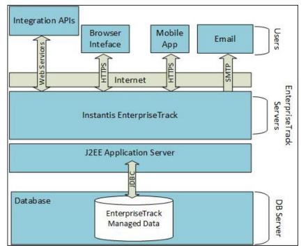
Oracle Instantis EnterpriseTrack resides on an application server. The application data repository resides on the database server. Typical Oracle Instantis EnterpriseTrack deployments consist of the following components:
