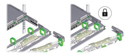
D Align connector C with the slide-rail so that the locking spring is positioned inside (server side) of the right slide-rail.
