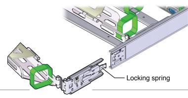
E Insert connector C into the right side-rail until it locks into place with an audible click
