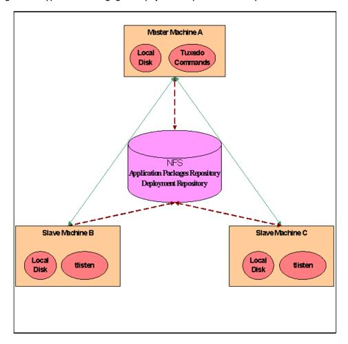
Figure 11-1 Applications Packaging and Deployment Component Relationship
