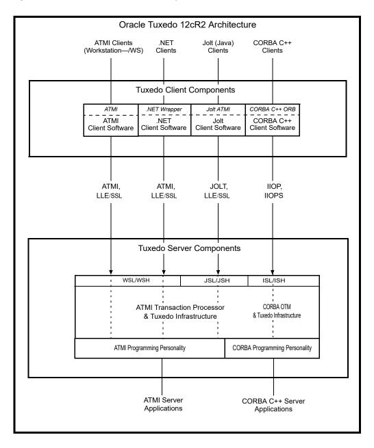
Figure 1-1 Oracle Tuxedo Client and Server Components
