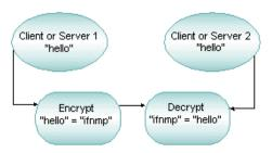
Encryption does not increase the number of bits in the data, but it adds processing time to the task of sending a message. Because data is compressed during encryption, however, lost processing time may be bought back, since less data is being sent across the network. When data is compressed, there is also a moderate boost to security, because the data is somewhat scrambled during compression.
