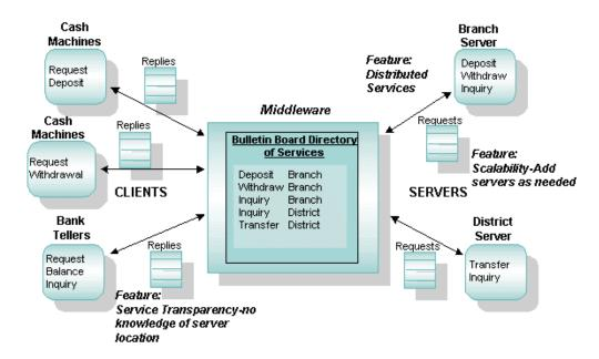
Figure 1-2 Clients and Servers in a Sample Banking Application
