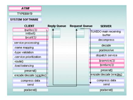
A client uses an ATMI function to request a service by name. A *naming* facility is used to check the MIB to determine whether the specified service is currently available.
