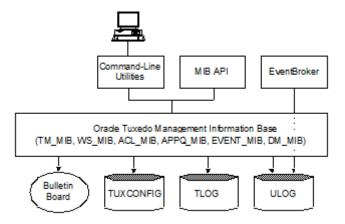
The Oracle Tuxedo MIB contains all the information necessary for the operation of an Oracle Tuxedo application. It contains the TM\_MIB, which is common to all applications, and the following component MIBs, each of which describes a subsystem of the Oracle Tuxedo system:
