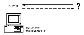
Any process that wants to be notified about a particular event (such as a machine being shut down for maintenance) can *register* a request, with the system, to be notified automatically. Once registered, a client or server is informed whenever the specified event occurs. This type of automatic communication about an event is called *unsolicited notification*.
