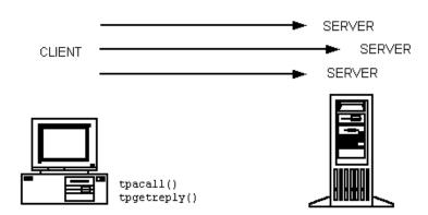
Figure 2-4 Asynchronous Request/Response Communication
