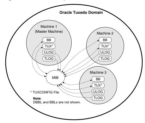
Figure 3-2 High-Level View of Oracle Tuxedo MIB Operation
