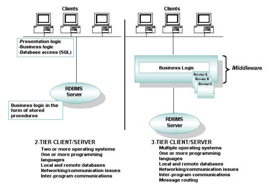
In 2-tier client/server applications, the business logic is buried inside the user interface on the client or within the database on the server in the form of stored procedures. Alternatively, the business logic can be divided between the client and server. File servers and database servers with stored procedures are examples of 2-tier architecture.
