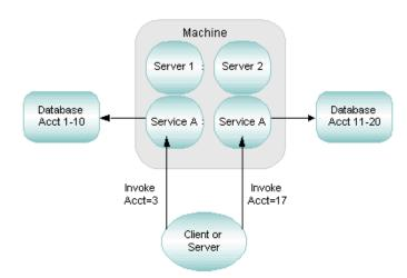
Figure 2-14 Data-Dependent Routing with a Horizontally Partitioned Database
