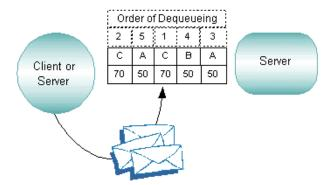
A request for service C is always dequeued before a request for A or B due to the higher priority of C. Requests for A and B have equal priority. This feature is useful in applications in which not all requests are equally urgent or important.
