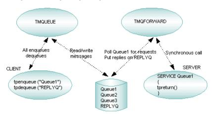
Figure 2-6 Storing and Forwarding Messages Using TMQFORWARD
