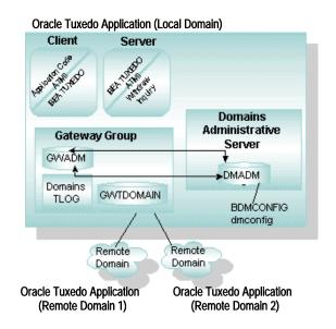
Figure 2-8 Interdomain Communication Using the TDomain Gateway Group
