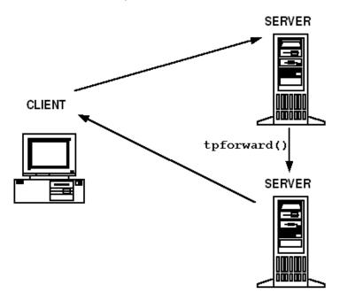
There is no limit to the number of times a request can be forwarded. Because a service that forwards a request does not need to wait for a reply from the service receiving the request, forwarding, unlike nesting requests, does not block servers. Forwarding, however, is not supported by the X/Open protocol X/ATMI, which may be a problem in some applications.
