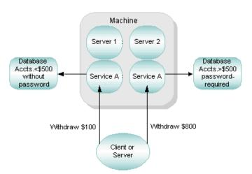
Figure 2-15 Data-Dependent Routing with Rule-Based Servers
