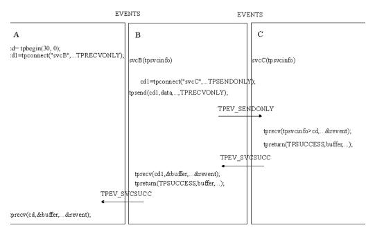
Figure 9-1 Connection Hierarchy in Transaction Mode
