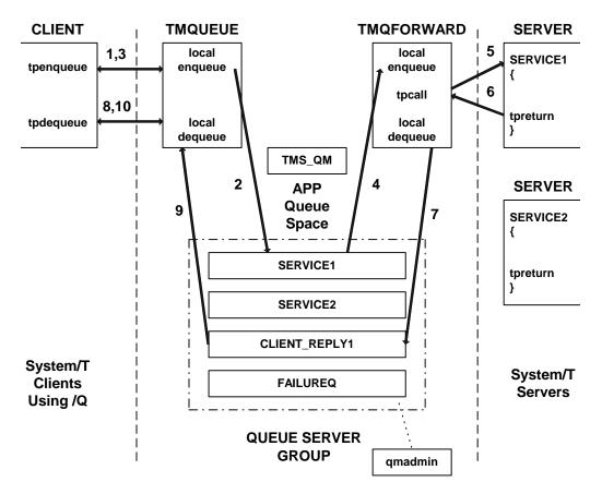
The figure illustrates how each component of the queuing system operates for queued service invocation. In this discussion, we use the figure to explain how administrators and programmers work with the Oracle Tuxedo /Q component to define it and use it to queue a message for processing and get back a reply. The queuing service may also be used for simple peer-to-peer communication by using a subset of the components shown in the figure.
