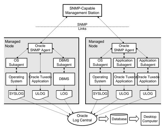
Oracle SNMP Agent provides the SNMP link from Tuxedo applications to SNMP-compliant network management frameworks (for example, HP OpenView) for monitoring, control, and alarm notification, as follows:
