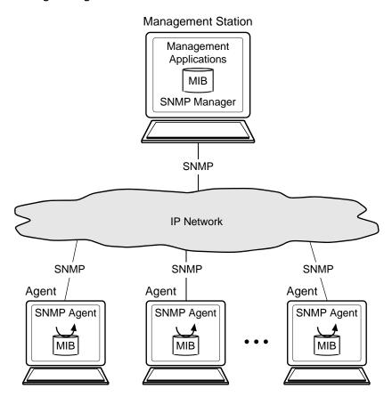
An SNMP-compliant MIB contains definitions and information about the properties of managed resources and the services that the agents support. The manageable features of resources, as defined in an SNMP-compliant MIB, are called *managed objects* or *management variables* (or just *objects* or *variables*).
