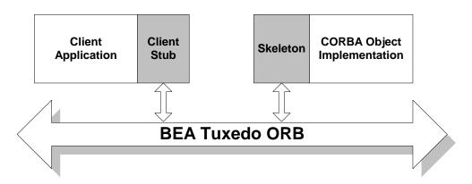
When a client application sends a request, the request is implemented as an operation on the client stub. When the client stub receives the request, the client stub sends the request to the Object Request Broker (ORB), which then sends the request through the Oracle Tuxedo system to the skeleton. The ORB interoperates with the TP Framework and the Portable Object Adapter (POA) to locate the correct skeleton and object implementation.
