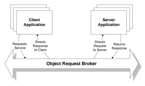
CORBA defines the ORB as an intermediary between client and server applications. The ORB delivers client requests to the appropriate server applications and returns the server responses to the requesting client application. Using an ORB, a client application can request a service without knowing the location of the server application or how the server application will fulfill the request.
