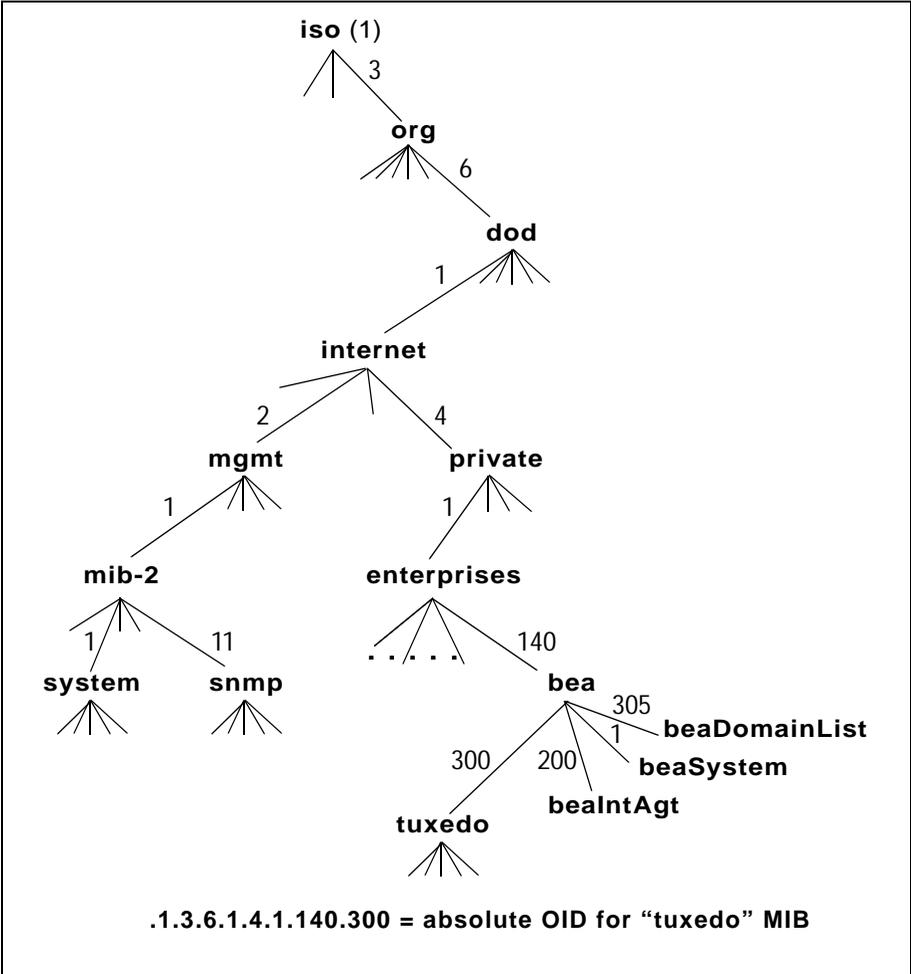
In this hierarchy, each Oracle private MIB object that the Oracle SNMP Agent software manages has a unique object identifier. A prefix of .1.3.6.1.4.1.140 points to the objects in the Oracle private MIB for the Oracle SNMP Agent software.
