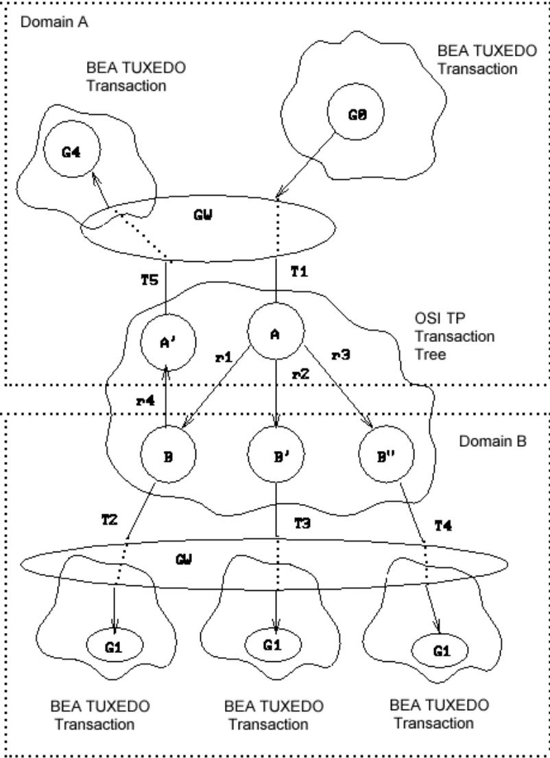
The TDomain instantiation provides a tightly-coupled integration that solves this deadlock problem by minimizing the number of transaction branches required in the interoperation between two domains. The corresponding transaction tree is shown in [Figure 4-6](#).
