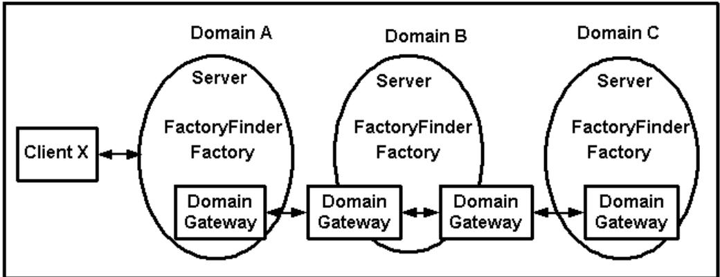
Domains A and B are directly connected, and Domains B and C are directly connected, but A and C are not directly connected. For Domains A and C to communicate, they must use Domain B as the intermediary. Therefore, the `DMCONFIG` file for Domain A must state that it is possible to connect to Domain C by going through Domain B (and vice versa). That is, the connectivity is:
