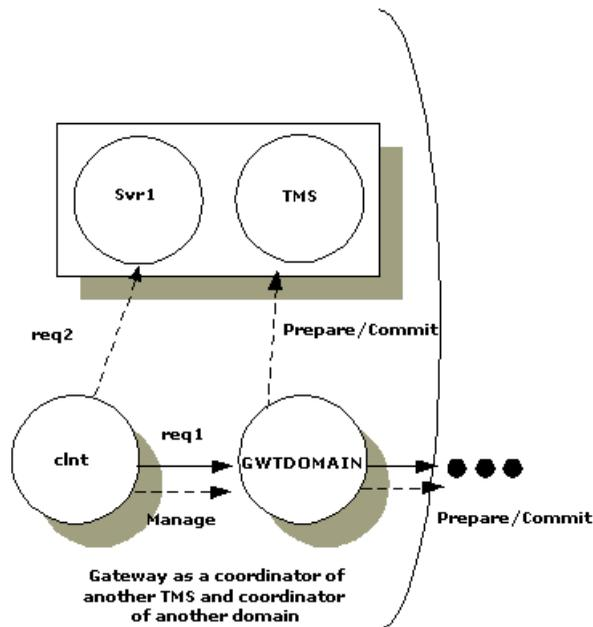
4. Gateways manage transaction commitment for a particular client or for a server that uses the forwarding service with the `AUTOTRAN` capability. When this combination is used, the last server in the forward chain (the domain gateway) issues the commit and becomes the coordinator of the transaction. (A domain gateway always acts as the last server in a forward chain.)
