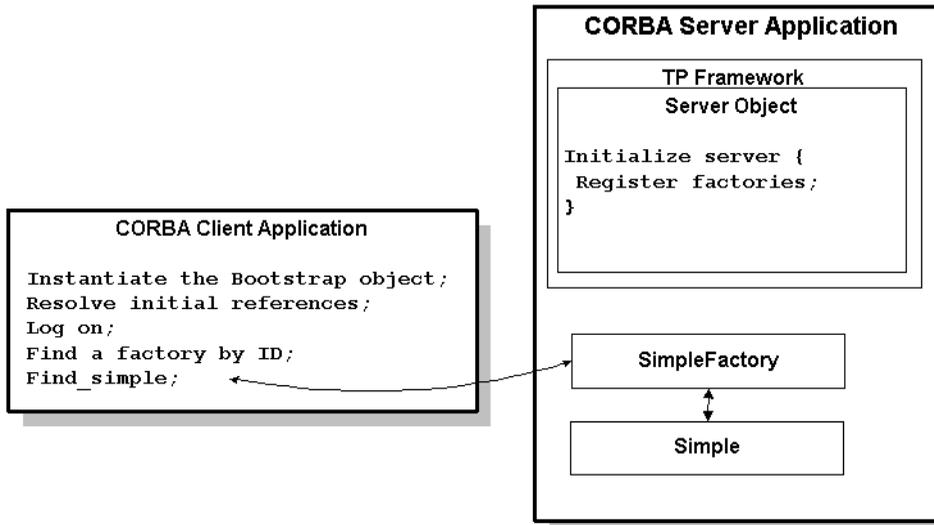
The SimpleFactory object then returns the object reference to the Simple object to the client application.
