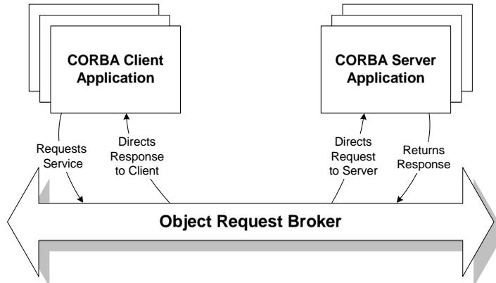
When the client application uses IIOP to send a request to the Oracle Tuxedo domain, the ORB performs the following functions:
