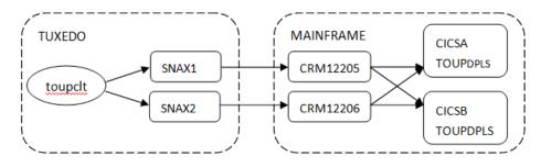
In this scenario, the load balancing / failover can be accomplished via following four paths:
