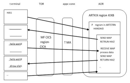
There is a TOR with terminals on mainframe, and an ART AOR on open system, they communicate each other via APPC connection provided by TMA SNA.
