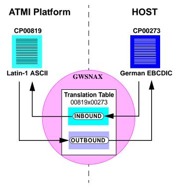
The figure demonstrates how an ATMI application using the Latin-1 ASCII code page CP-00819 character set operates with a host application using German EBCDIC code page CP-00273. The Oracle Tuxedo Mainframe Adapter for SNA translation table 00819x00273 provides both the inbound and outbound conversions.
