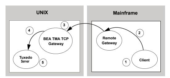
Figure 3-2 Security Checking for Mainframe to UNIX Transactions
