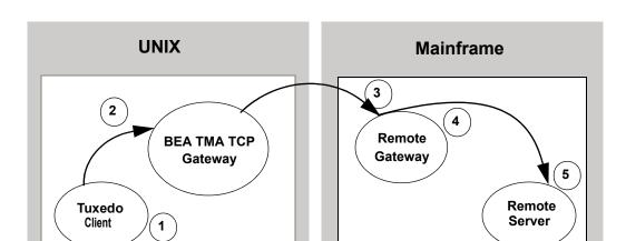
Figure 3-1 Security Checking for UNIX to Mainframe Transactions
