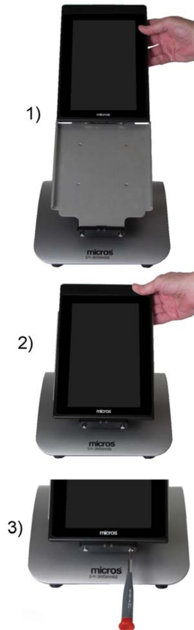
Figure M.5: Installing the mTablet in mStation - Portrait Mode The mTablet orientation may be changed to the Landscape position by depressing the Rotate Button behind the slide tray.
