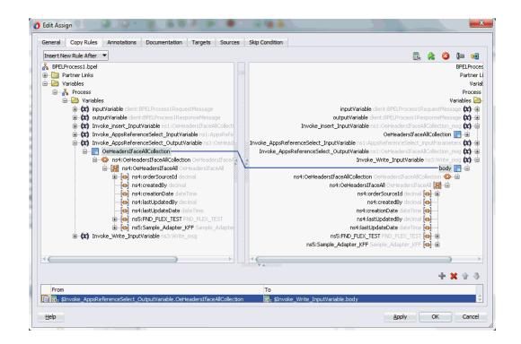
Since the OeHeadersIfaceAllCollection node variables contained in the Source and Target are identical, instead of specifying each flexfield, we can simply drag the source node (OeHeadersIfaceAllCollection) to connect to the target node (OeHeadersIfaceAllCollection) to complete the second **Assign** activity.
