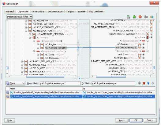
Use **Assign** activity to provide input payload information to the TCA Location object of the target parameter.
