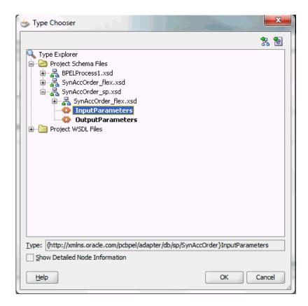
Click **OK**. The selected SynAccOrder\_sp.xsd schema is displayed as URL and InputParameters is displayed as Schema Element.
