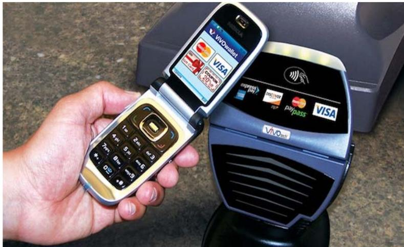
The discount is applied immediately to the check without interrupting the cashier. When tapped, the ViVOPay 4800 will beep and its lights will flash, indicating a receipt from the phone. After accepting the discount, POS Operations will display 'Discount sent by customer' in the POS.
