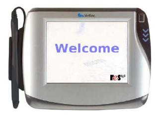
The MX870 functions as an extension of the workstation in order to make ringing transactions more efficient. During a transaction, the operator will ring items into their workstation. The MX870 will display items as they are rung, and will prompt the customer when their input is required.
