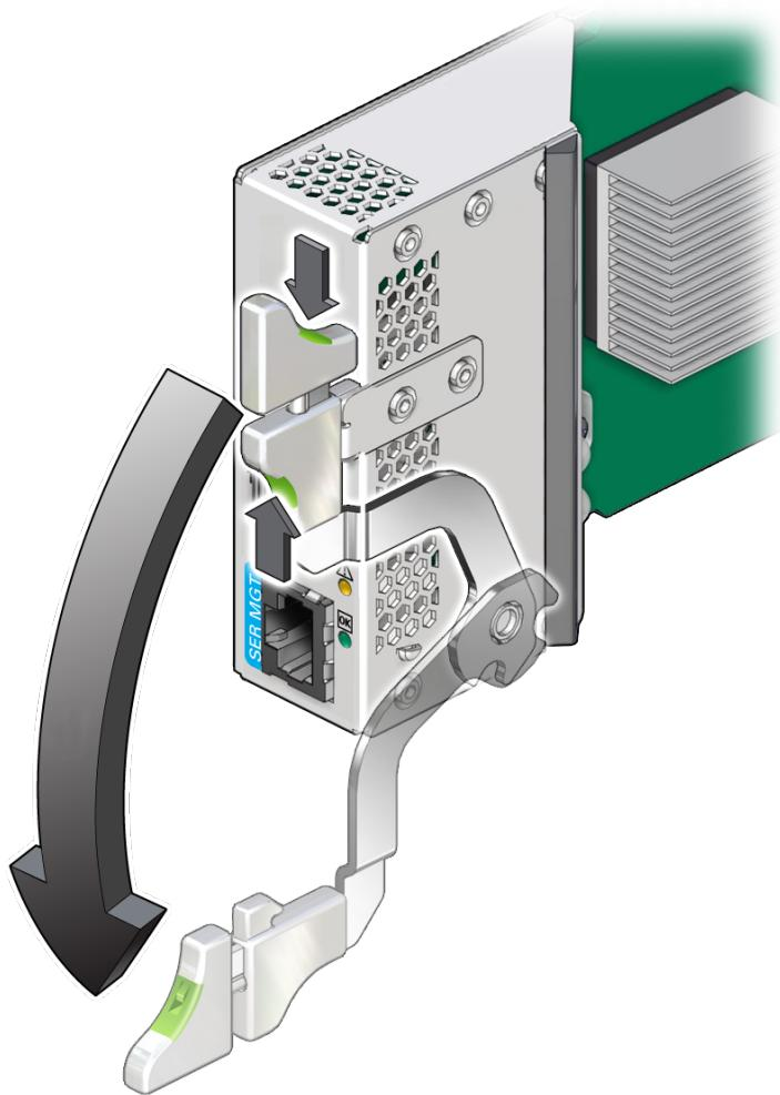
5. Align the module to the slot where you are installing it.
