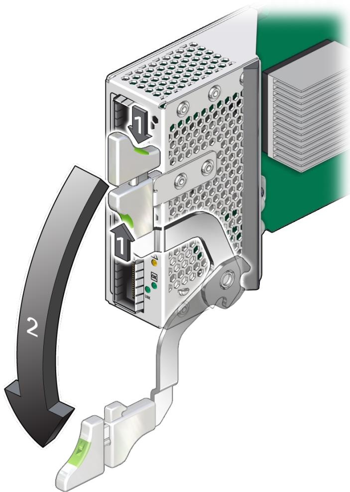
6. Align the module to the slot where you are installing it.
