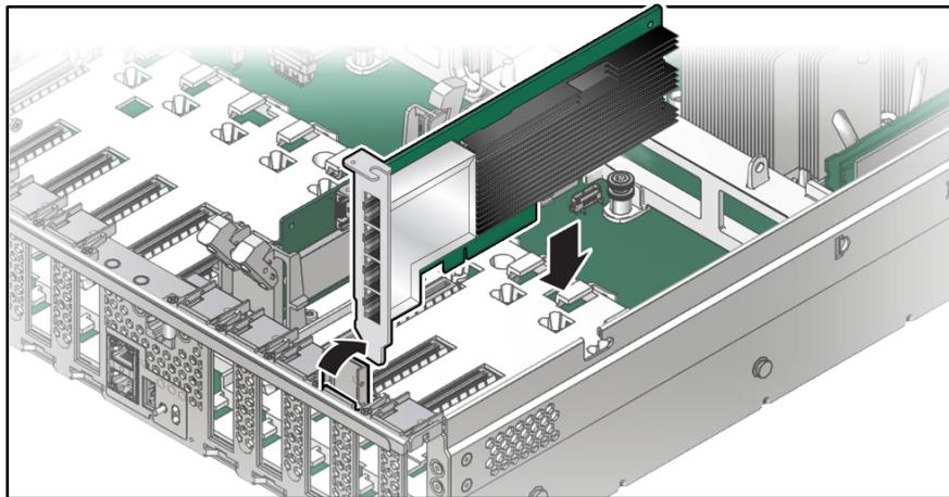
7. **Slide the adapter face plate into the small slot at the end of the PCIe opening.**
