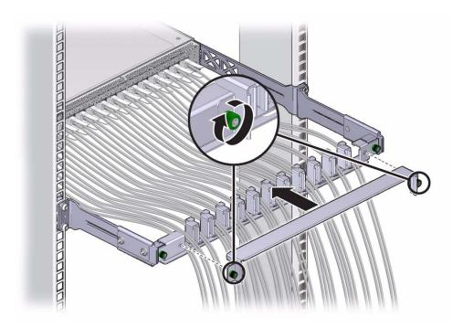
12. Route the InfiniBand cables so that they do not interfere with other cables, or with servicing the switch or other systems.
