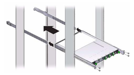
9. Mount the front of the switch chassis to the front rack posts with two captive nuts and two screws at each side.
