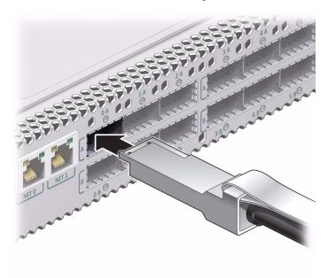
**Note** – On some QSFP cable connectors, there is a retraction strap. Both the retraction strap and L groove indicate the reference surface for the connector. When installing QSFP cables in the top row of receptacles (0A, 1A, 2A, and so on), ensure that the L groove and retraction strap are up. When installing QSFP cables in the bottom row of receptacles (0B, 1B, 2B, and so on) ensure that the L groove and retraction strap are down. Refer to *Switch Service*, identifying the InfiniBand cable.
