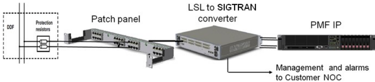
Figure 59 – LSL/HSL to SIGTRAN Converters – connectivity
