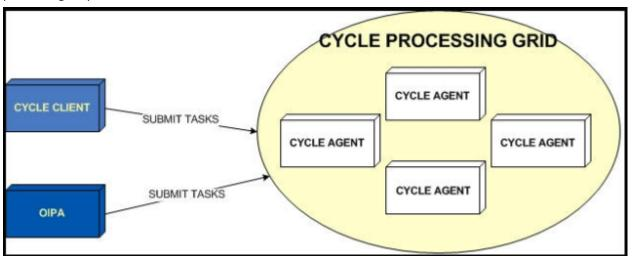
Cycle Agents are the programs that execute the tasks that comprise the Cycle batch process. Each Cycle Agent runs in its own Java Virtual Machine (JVM). Depending on the number of tasks that must be executed during Cycle processing, any number of JVMs may be used to run the desired number of Cycle Agents. The JVMs may be started on one or more physical machines. If more than one machine is used, they will be effectively clustered via the Coherence clustered caching and messaging system.
