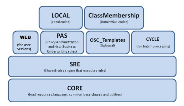
OIPA caches static configuration data and other data that rarely change. There are seven cache regions in the system, each for a different module. Every cache region is configured separately, allowing each one to be configured differently.
