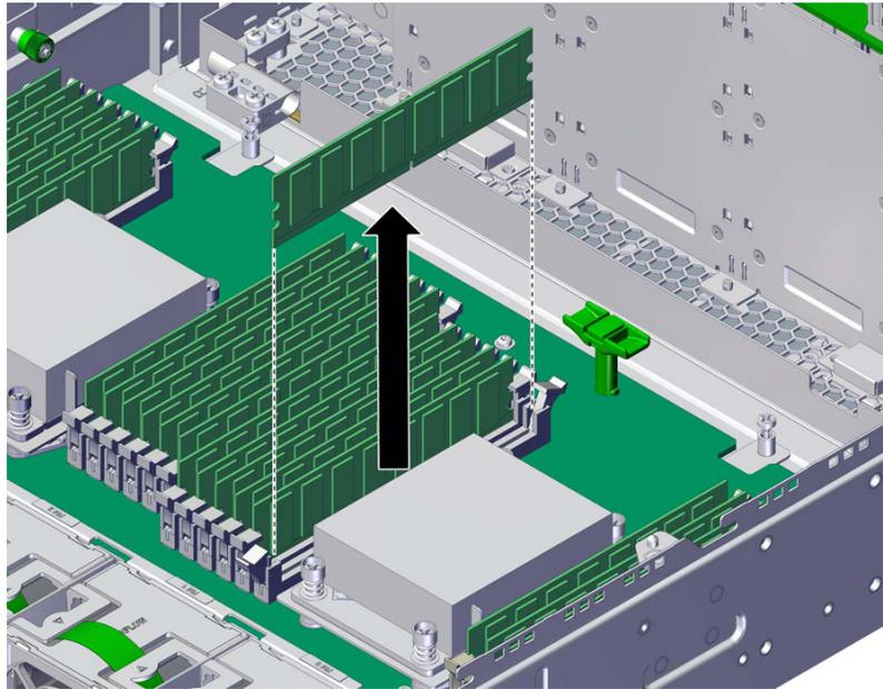
9. Align the replacement DIMM with the chassis slot.
