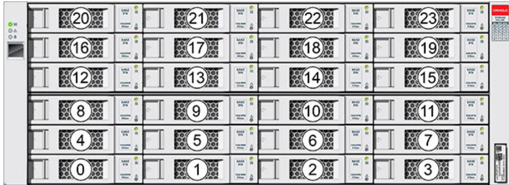
Read cache devices cannot be installed in the Sun Disk Shelf.
