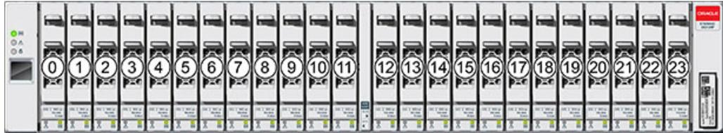
Up to four write-optimized log SSDs are supported per disk shelf. Log devices should be populated in order of slots 20, 21, 22, and 23.
