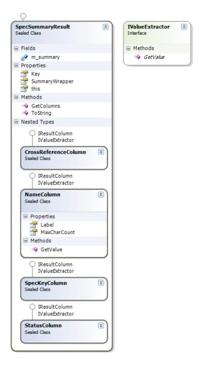
SpecSummaryResult also contains internal classes for each column: each implements the IResultColumn interface, providing the Label property for the column name, and the MaxCharCount for the length. Additionally, each internal ResultColumn class implements a GetValue() method from a new interface called IValueExtractor that provides the value to display for each result.
