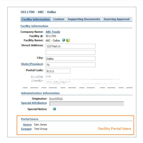
To view the Portal Users section on an SCRM facility profile, make sure the following configuration entry is set to true: CustomPortal.SCRMFacility.Participants.Enabled
