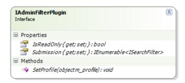
The SetProfile method is used to pass in the Custom Portal Profile object, which can then be used to save the Search Filter values to the Profile via the Profiles. SetSearchFilter method. The Search and/or Rendering Plugins can later retrieve these Admin Search filters directly from the Profile.
