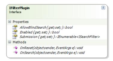
The Submission property is used to get and set the search filters. The search filters are retrieved from the form's data entry fields, and are then passed into the Search Plugin.
