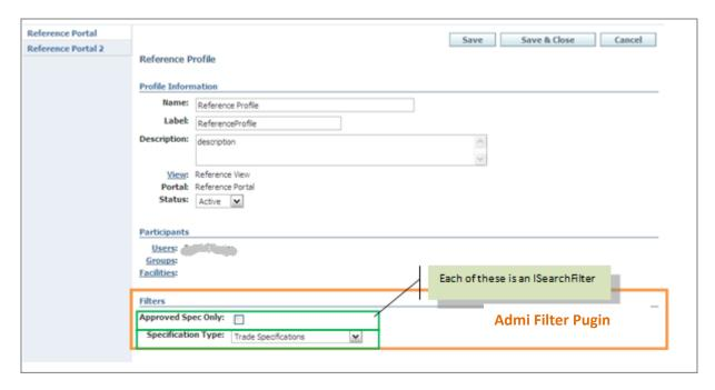
The IAdminFilterPlugin is typically implemented as a user control, using data entry fields to set each ISearchFilter.
