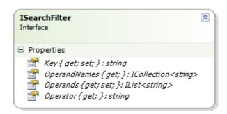
A simple example of using a SearchFilter would be to filter the results based on specification type. Setting the Key="SPECTYPE" and the Operands to a list of desired spec types (ex: ingredient, trade). The SearchPlugin would then use the filters and filter out specs that were not of the correct type.
